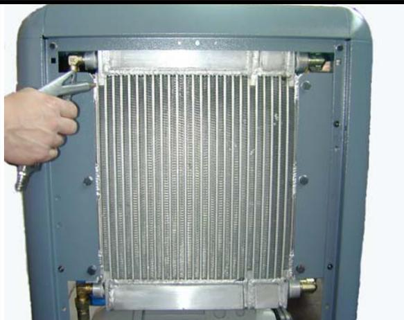
A close-up photograph showing a person's hand holding a silver air hose nozzle. The nozzle is directed towards the vertical fins of a metal radiator, which is part of a larger blue-grey machine. The radiator is mounted on a metal frame. The background is a plain, light-colored surface. |
